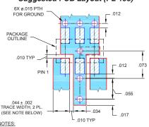
TRACE WIDTH IS SHOWN FOR ROGERS RO4350B WITH DIELECTRIC THICKNESS .020° ± .0015°. COPPER: 1/2 OZ. EACH SIDE. FOR OTHER MATERIALS TRACE WIDTH MAY NEED TO BE MODIFIED.
